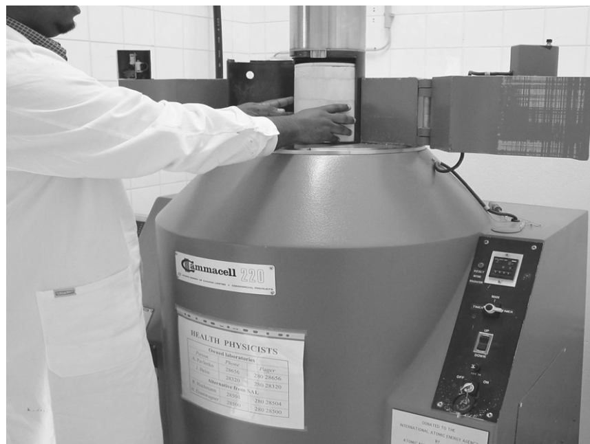
Figure 1. In preparation for irradiation, a canister of insects is placed in the irradiation chamber (while it is in the shielded position) of a self-contained gamma irradiator. Depending on the dose rate of the day, the timer on the control panel (bottom right) is set to give the desired dose.
